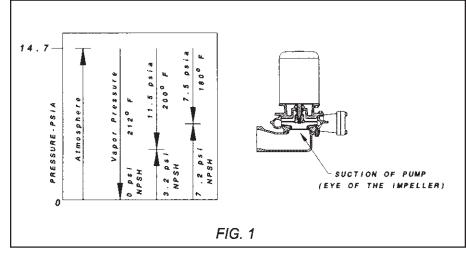
200°F is 11.5ps, so 14.7 - 11.5 = 3.2psi NPSH. It is conventional to express NPSH in FT. of water and as 1psi = 2.31 FT., then 3.2psi X 2.31  $^{\text{FT}}$ /psi = 7.39 FT. In a similar example, the vapor pressure for 180°F is 7.5psi, so the NPSH equals 14.7 - 7.5 = 7.2psi, then 7.2psi X 2.31  $^{\text{FT}}$ /psi = 16.63FT. NPSH (Fig.1).
